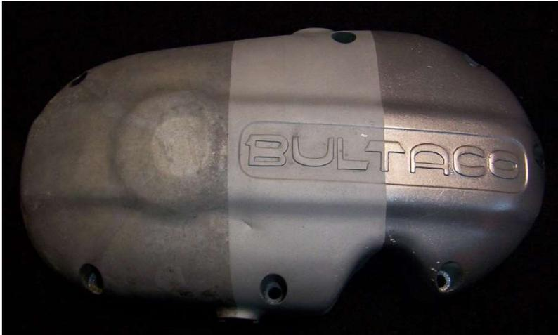
Difference between an original weathered finish, dry media blasting and a vapor blasted finish.
